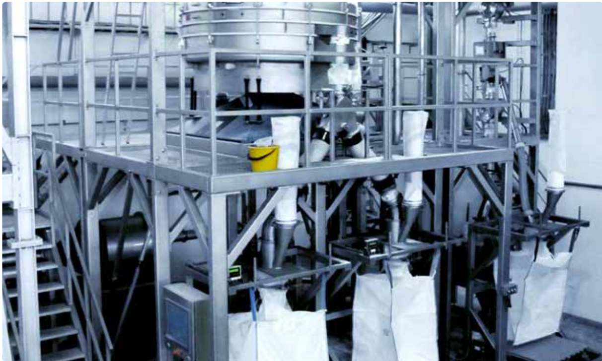
REKORD C grinding plant for food grade phosphates
