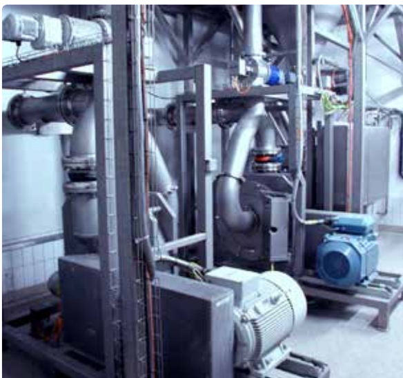
REKORD 630 GMP fine grinding plant for lactose
